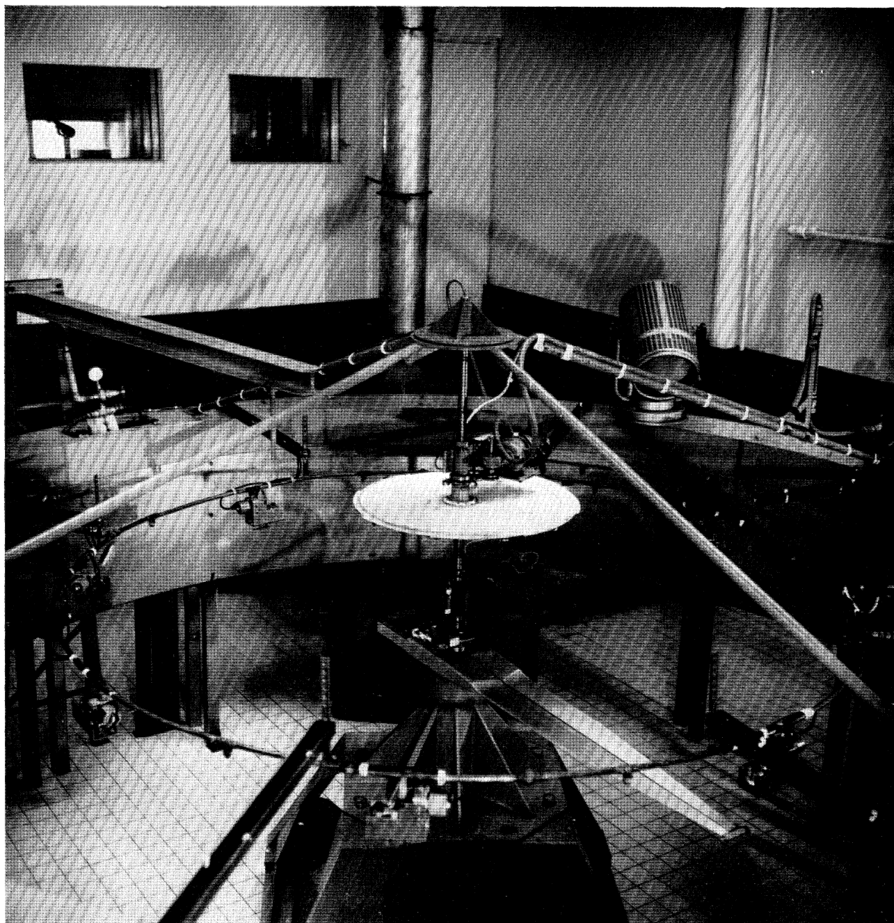
FIGURE 1. Whirling arm equipment for testing rain erosion behaviour.
